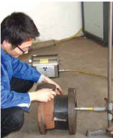
Gama ray fault detection of Non-destructive testing
