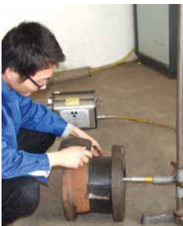
Gama ray fault detection of Non-destructive testing
