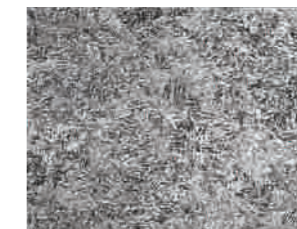
Figure 2: Acceptable microstructure after welding. (100X) (1)
