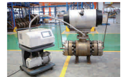
Low Fugitive Emission Test
