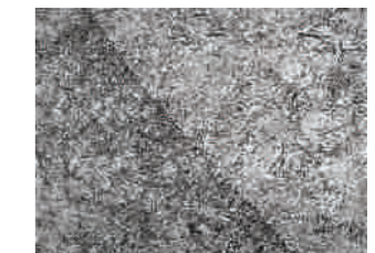
Figure 3: Acceptable microstructure in heat affected zone. (100X) (1)
