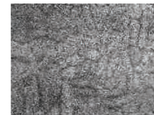
Figure 1: Acceptable microstructure of castings (100X) (1)
